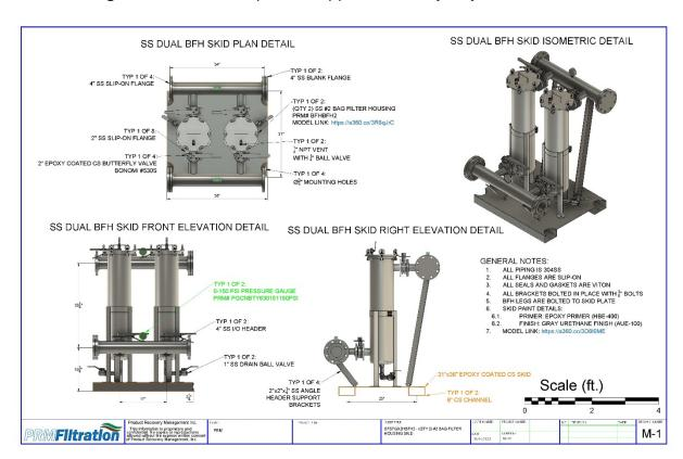
PRM #2 Size Dual Bag Filter Housing Skid, 4 Inch Flange In/Out; 150 psi
